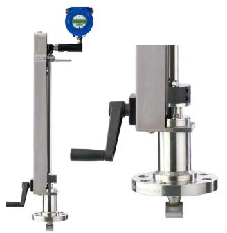
Insertion vortex flow meters detect the frequency of alternating low pressure vortices that are formed as flow is diverted around a bluff body. These swirling low pressure zones apply lateral pressure first to one side and then to the other of sensors located downstream of the bluff body. This causes the sensors to vibrate. The frequency of this vibration is directly proportional to the flow velocity.
