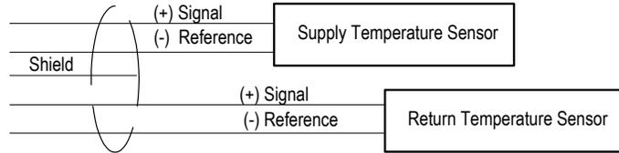
1000 OHMS 4-WIRE PLATINUM RTD TEMPERATURE INPUTS
