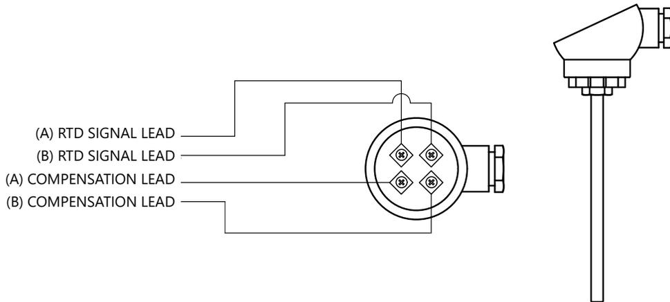
Refer to Temperature Sensor Connection on next page for additional details on the terminal location.
