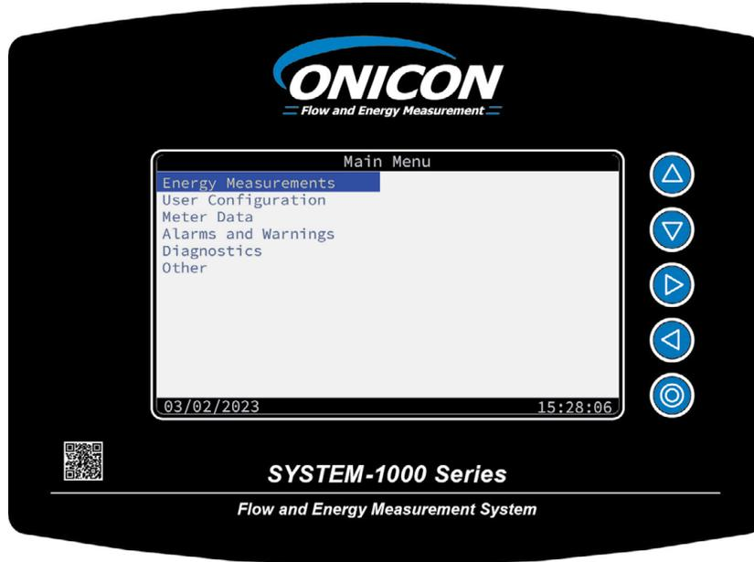
The main menu screen will indicate the meter is operating. Press the Energy Measurement screen to access the real-time data.
