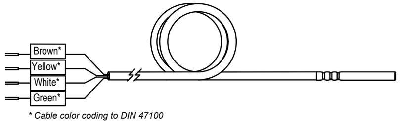
1000 OHMS 4-WIRE PLATINUM TEMPERATURE INPUTS
