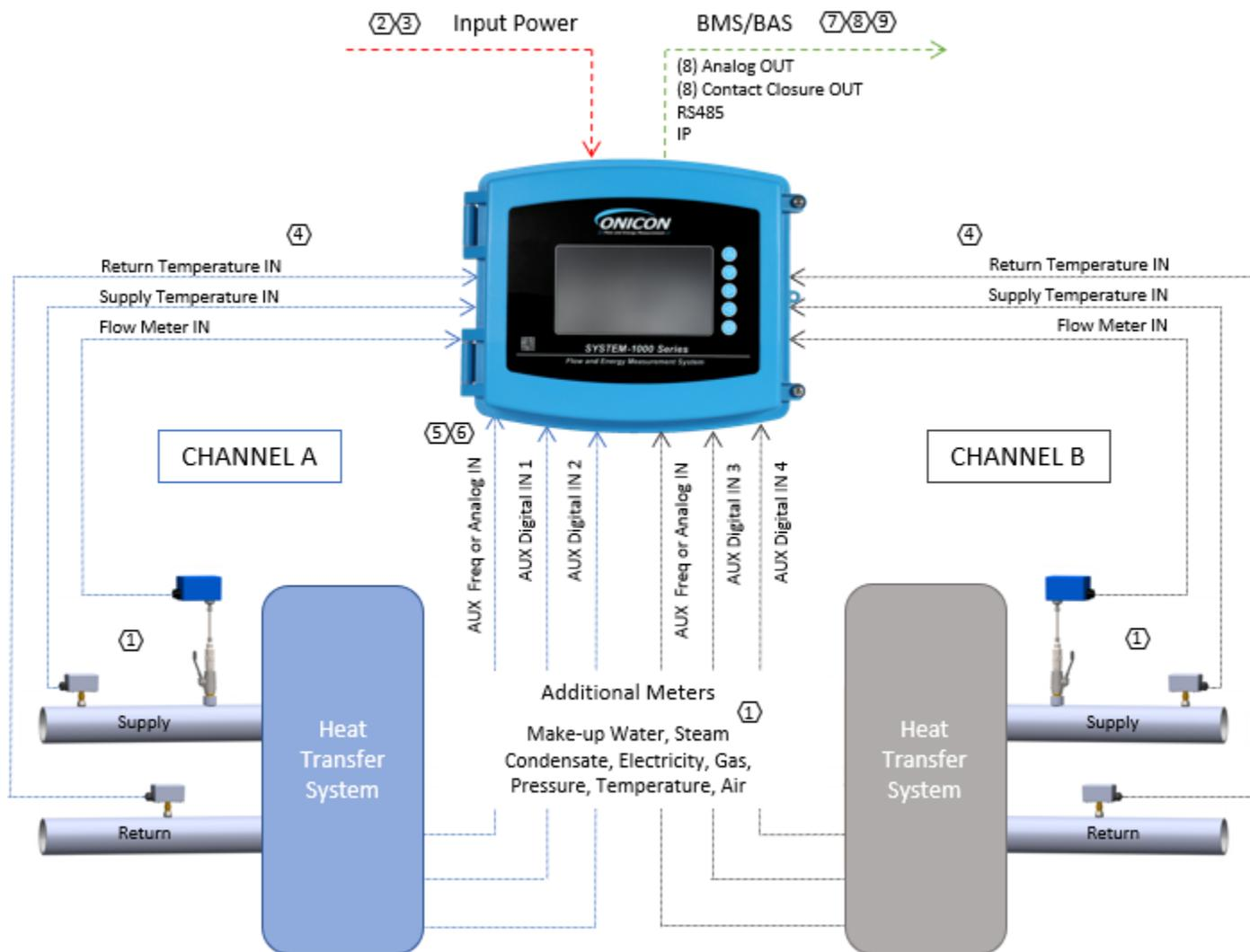
1. ONICON Flow Meters and Temperature Sensors are provided separately
