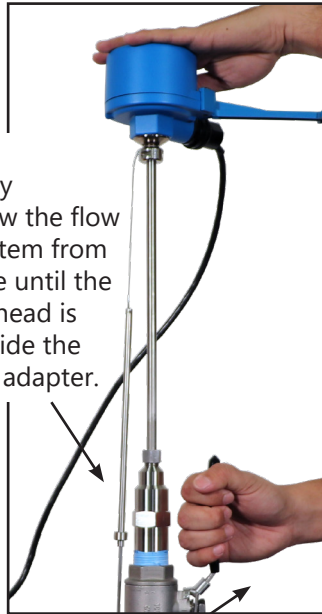
Step 3: After the meter is completely withdrawn, slowly close the valve to isolate flow.
