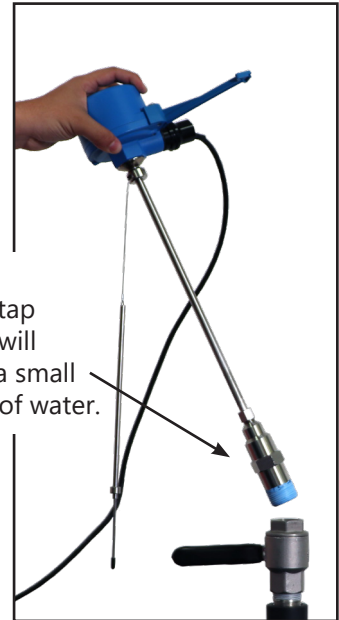
Step 4: After the valve is completely closed, unscrew the hot tap adapter from the valve. For hot water meters, partially unscrew the adapter to vent pressure before fully removing the meter.
