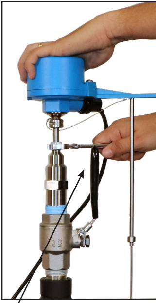
Step 1: Slowly loosen the position clamping nut while maintaining a firm grip on the enclosure to counteract the effect of pressure in the pipe.
