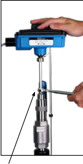
Step 1: Slowly loosen the position clamping nut while maintaining a firm grip on the enclosure to counteract the effect of pressure in the pipe.
