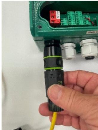
B. Loosen the barrel cover to expose the RJ-45 coupler. (Again, do not allow the coupler to rotate).
