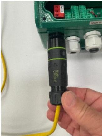
A. Loosen the strain relief nut completely and slide down the existing cable (if applicable). Note: Do not allow the entire coupler to rotate.
