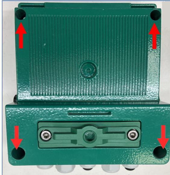
3. Carefully detach the front panel, (note ribbon cable connection).
