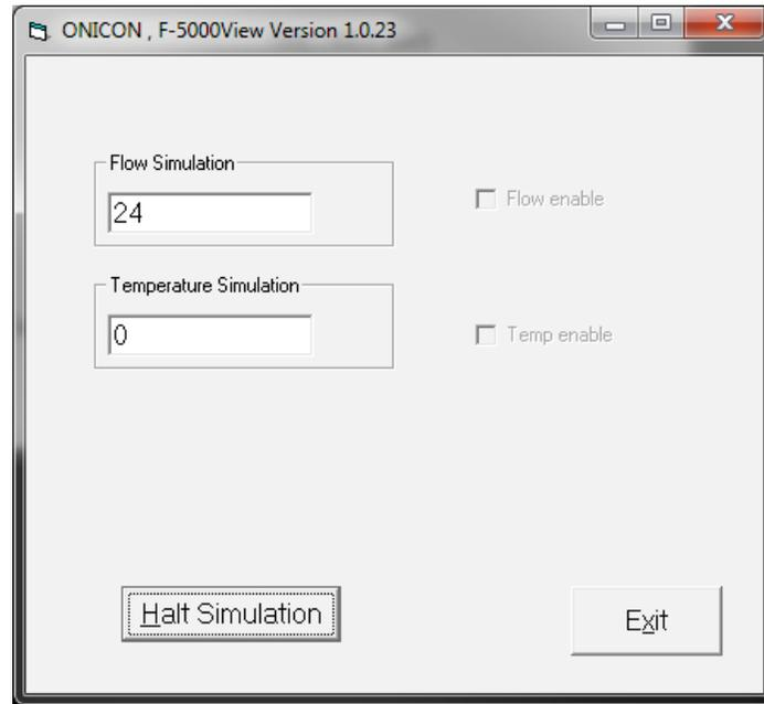
In Simulation mode, all F-5000 outputs and the Totalizer respond as if in normal measurement mode. Click "Halt Simulation" to end.
