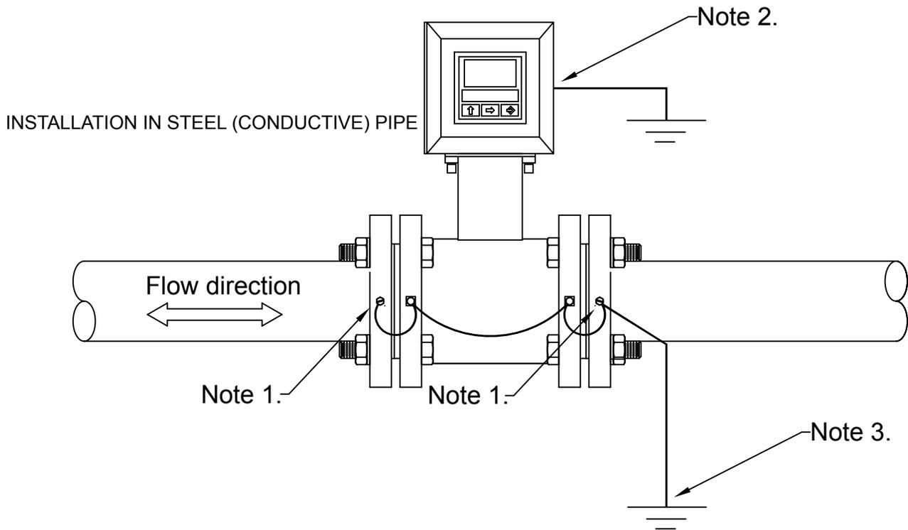
**Note 1.** Using a #21 (0.159") drill bit, drill a ½" deep hole in edge of each mating flange. Tap each hole using a 10-32 tap. Secure the ring connectors (provided) and grounding wires to the flange using the green grounding screws (provided).
