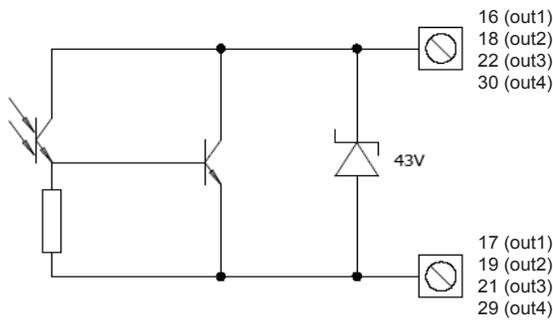
Opto-coupled open collector pulse outputs
