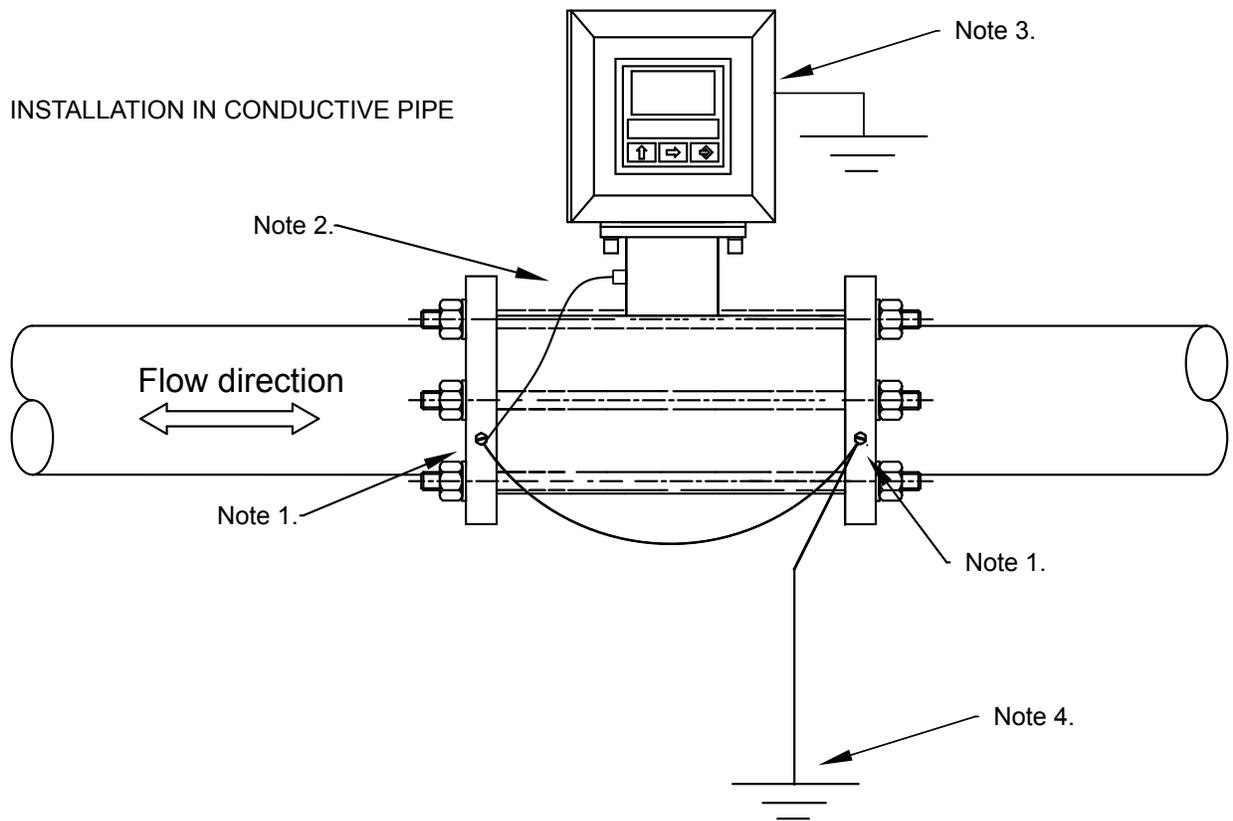
**Note 1.** Using a #21 (0.159") drill bit, drill a 1/2" deep hole in edge of each mating flange. Tap each hole using a 10-32 tap. Secure the ring connectors (provided) and grounding wires to the flange using the green grounding screws (provided).
