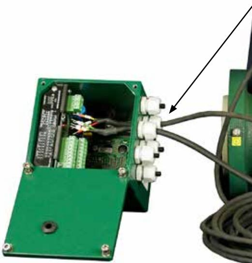
Connect the coil and electrode wires to the appropriate terminals according to the numbered tags on each wire.
