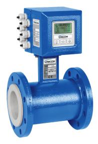
Faraday's Law states that a voltage will be induced in a conductor (the conductive fluid) when it passes through a magnetic field (generated by the meter), and that voltage will be directly proportional to the velocity of the conductor (the fluid). This voltage is measured by electrodes on opposite sides of the flow tube and used to calculate the flow velocity.
