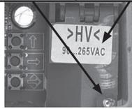
**Step 5: Pull straight out on the connector to remove it.**
